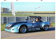
Webers. Griffin radiator. Aluminum fly wheel - Tilton clutch. ATL cell. 8-point cage. Adjustable aluminum shocks and adjustable sway bars. Wilwood brakes,
